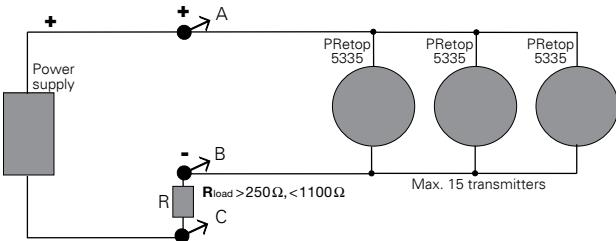
The outputs of max. 15 transmitters can be connected in parallel for a digital HART® communication on 2-wires.
