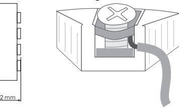
Wires must be mounted between the metal plates.
